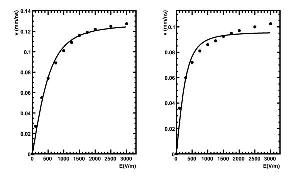
Figure 6.2: Drift velocities as a function of electric field for (left) electrons and (right) holes along the [100] axis in germanium with corresponding model calculations for a HPGe detector [91].
