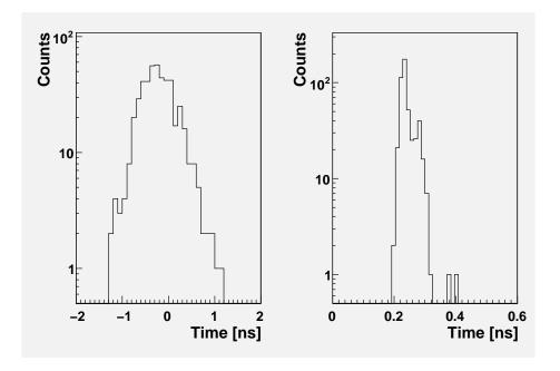
Figure 6.3: (left) The mean delay of signals for segments in SeGA and (right) the standard deviation of the delay for events in a given channel [89].
