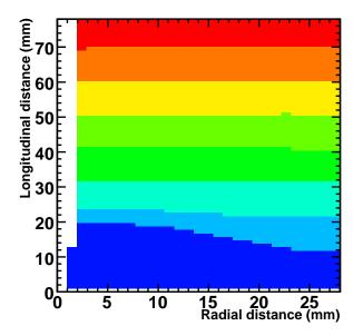
Figure 6.5: Segment division in a SeGA detector for a r-z plane based on the drifting of holes to a given electrode. The longitudinal distance is measured from the "A" segment (0 mm) to the "H" segment (80 mm).
