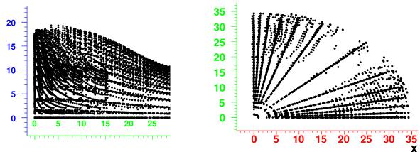
Figure 6.6: Calculated grid points for an "A" segment of a SeGA detector in the x-z plane (left) and x-y plane (right) which sample the segment volume to maximize the sensitivity to the changing shape of the waveform.
