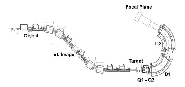
Figure 2.1: Schematic of the S800 spectrograph.
