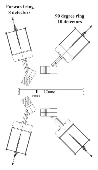
Figure 3.4: The setup used for the  $\alpha$ - $\gamma$  coincidence measurements to determine the polarization sensitivity.
