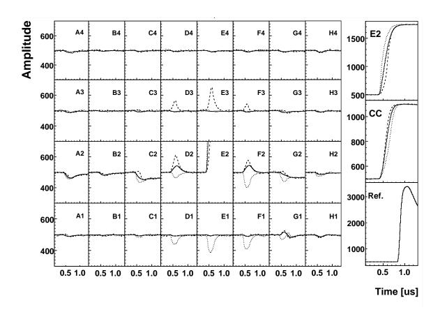
Figure 6.1: Induced signals recorded in the 32 segments and central contact of a SeGA detector for several events where a 1332 keV gamma ray from  $^{60}$ Co interacts in single segment E2 at different positions.  $\gamma$ - $\gamma$  coincidences are recorded in a CsF detector; this serves as a timing reference for the measurement [89].
