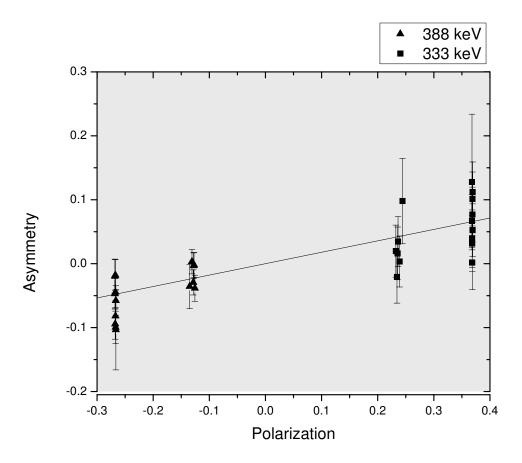
Figure 3.9: The asymmetry observed in the SeGA detectors for gamma rays of four known polarizations adjusted for the relative analyzing power of the Compton effect for the two different energies.
