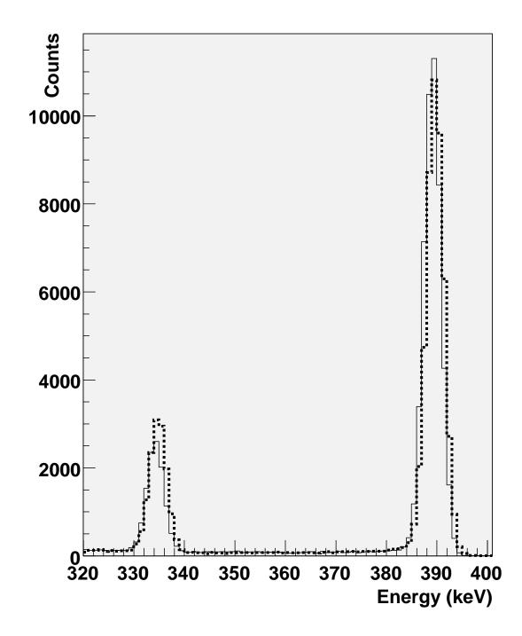
Figure 3.5: Gamma-ray spectrum for a detector in the forward (solid) and backward (dashed) rings in SeGA for the two gamma ray transitions in the  $^{245}\mathrm{Cm}$  following the  $\alpha$  decay of  $^{249}\mathrm{Cf}$  showing the difference in the angular distribution.
