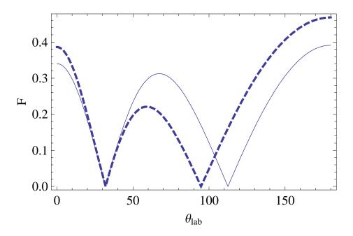
Figure 6.7: Angular distribution sensitivity for residues with  $\beta = 0.4$  (solid) and  $\beta = 0.525$  (dashed) considering placement of a second ring with the first ring fixed at 32°.
