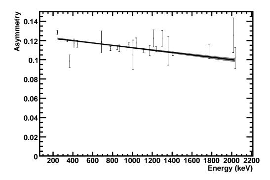
Figure 3.8: Geometric asymmetry measured for detectors in the forward ring for a range of energies for unpolarized gamma rays emitted from a  $^{152}$ Eu source. Included is a linear fit and error band.
