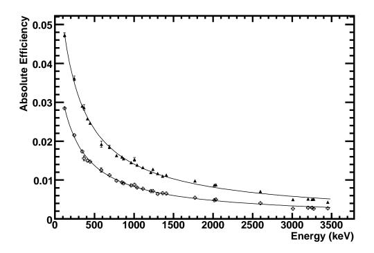
Figure 3.2: SeGA efficiency in the  $37^{\circ}$  ring (crosses) and the  $90^{\circ}$  ring (triangles) with associated fits in the form of Eq. 3.3.
