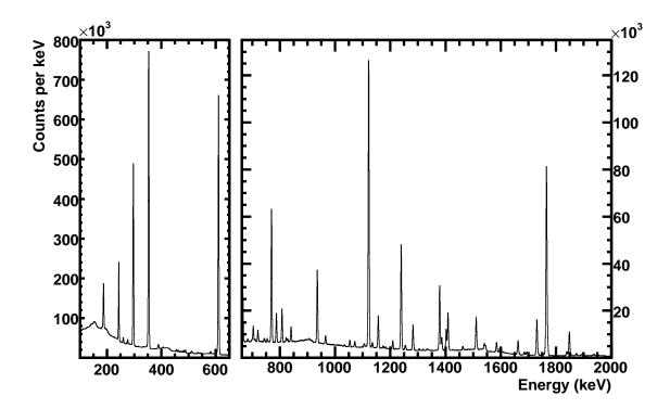
Figure 3.1: Calibrated <sup>226</sup>Ra energy spectrum of all 16 SeGA detectors summed.
